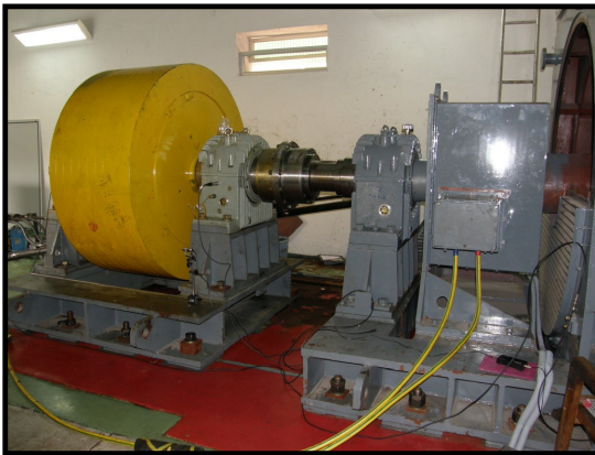
Vibration studies and on-site balancing of motor-generator-flywheel assembly. Weight of the flywheel was 16 tons and runs at 1500/1800 rpm. This machine was first of its kind developed in India for short circuit testing and analysis.
