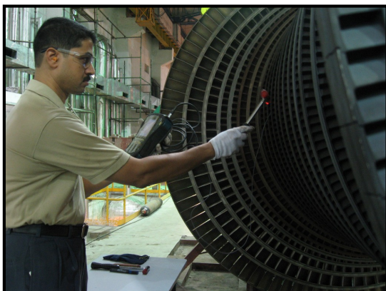
Natural frequency studies on 61.5 MW turbine rotor blades at Abhijeet Power site
