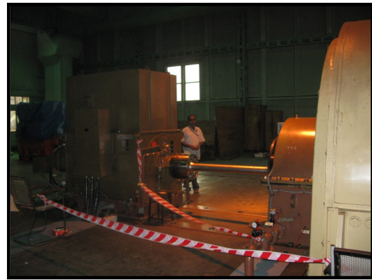
Vibration studies and on-site balancing of 2300 KW motor assembly (Alstom make) coupled to 54 ton generator assembly
