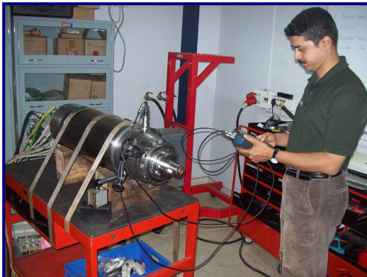
Vibration measurements and on-site balancing of high speed spindle assembly (25000 rpm)
