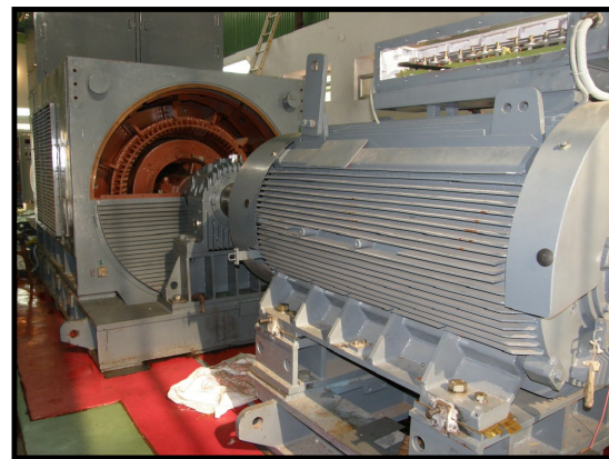
Vibration studies and on-site balancing of motor-generator-flywheel assembly. Weight of the flywheel was 16 tons and runs at 1500/1800 rpm. This machine was first of its kind developed in India for short circuit testing and analysis.
